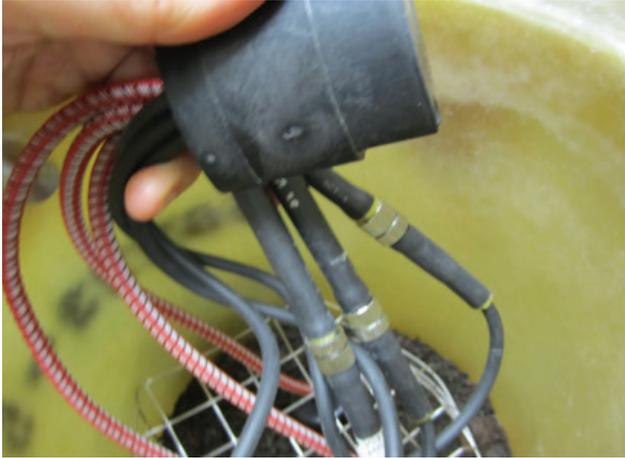
Secure the cable loops with the fastening straps, and place on the wire cage. Gently position within the center portion of the wire cage maintaining vertical loop orientation and minimizing cable extension outside the wire cage.
