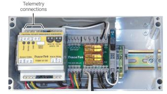
Figure 6. Telemetry Connections
