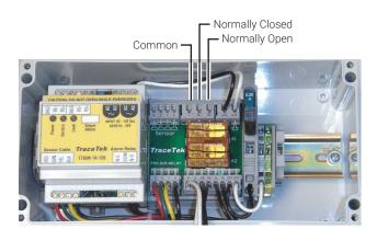
Figure 5. Alarm Relay Connections
