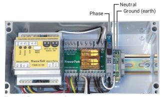
Figure 3. Power connections
