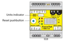
Figure 11. RESET pushbutton and units indicator locations
