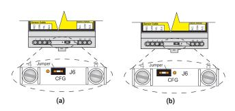
Figure 8. CFG jumper position for configuration mode (a) and normal operation (b)
