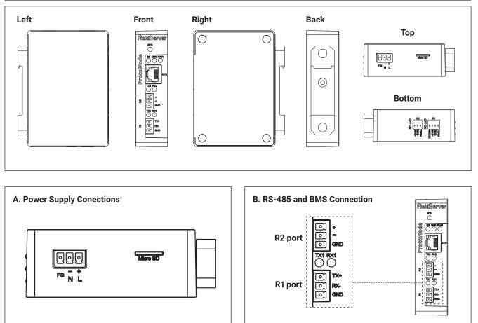
R1 port: RS-485 connection to nVent RAYCHEM controller. R2 port: RS-485 connection to BACNet MS/TP or Metasys N2. Ethernet port: BACNet IP connection.
