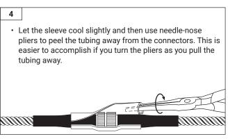
After removing the oversleeve, the male spinner on the metal connector may stick to the residual adhesive. Pliers can be used to free the spinner ring and separate the connector pair.
