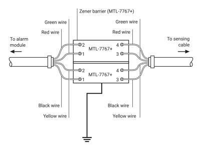
IMPORTANT: Hazardous Area approvals are carried by the barrier manufacturer. In order to achieve the necessary level of protection, the barrier manufacturer's instructions must be followed exactly.
