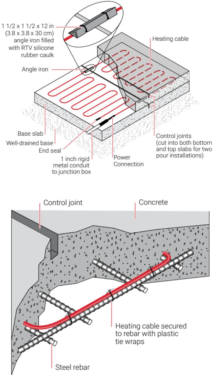
**Figure 2: Control joint**
