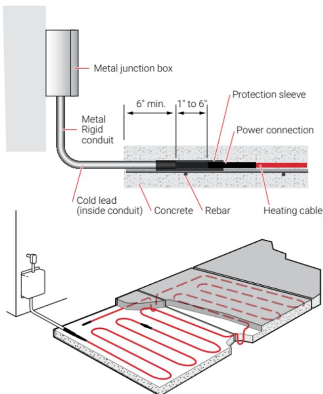
**Figure 3: ElectroMelt installation**
