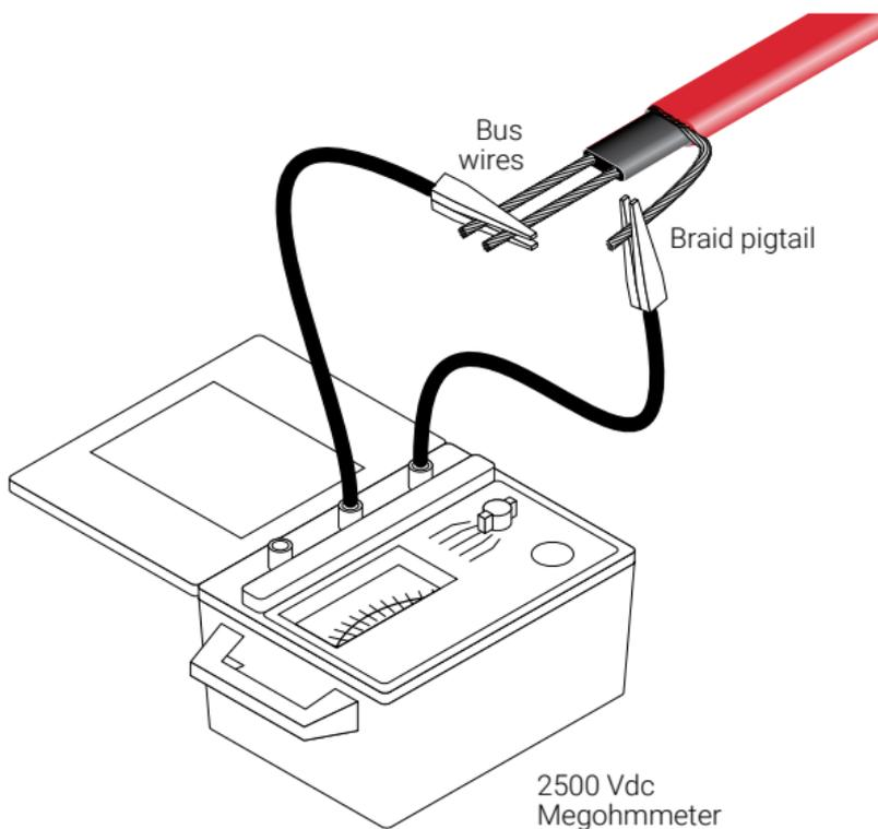
**Figure 7: Insulation resistance test**
