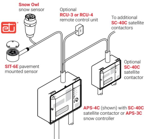
**Figure 4: Automatic snow melting control system**
