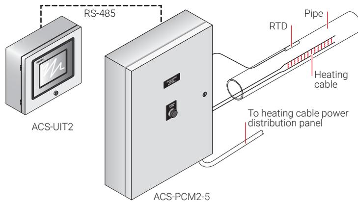
**Fig. 6 Typical configuration for the ACS-30 system**
