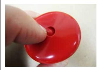
Push the TraceTek cable through the hole. You may need to bend the end cap to open the hole enough for the cable end to pass through.
