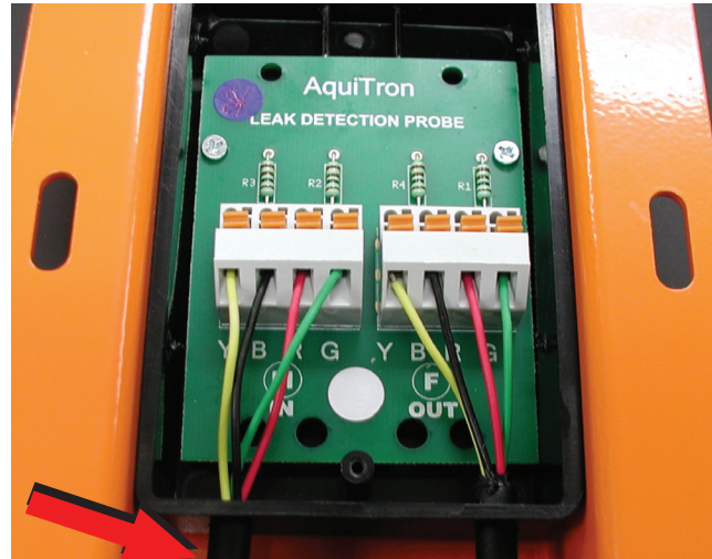
Figure 3. Multiple probe wiring configuration and suggested tie wrap location
