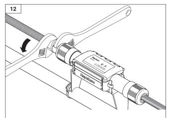
Using two wrenches, attach user-supplied 1/2-inch conduit. To avoid breaking housing, do not exceed 15 ft-lbs of torque. Broken connectors must be replaced.
