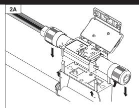
• For the RayClic-PC power connection, fold up the four outer snaps, then position the connector over the snaps and press down.
