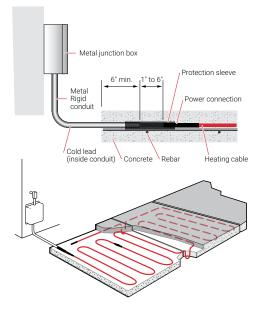
Figure 3: ElectroMelt installation
