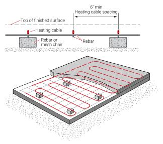
Figure 4: ElectroMelt installed on rebar
