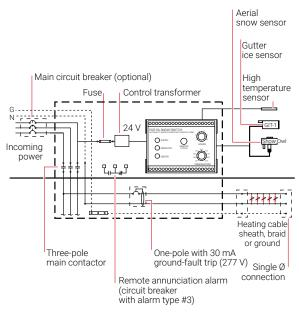
Figure 6: SMPG wiring diagram
