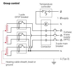
Figure 5: Typical controller wiring-multiple circuits
