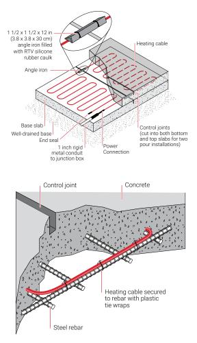
Figure 2: Control joint
