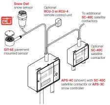
Figure 4: Automatic snow melting control system
