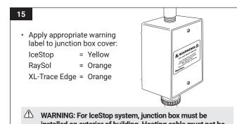
WARNING: For IceStop system, junction box must be installed on exterior of building. Heating cable must not be installed inside building, in conduit or under any form of insulation to minimize risk of fire.
