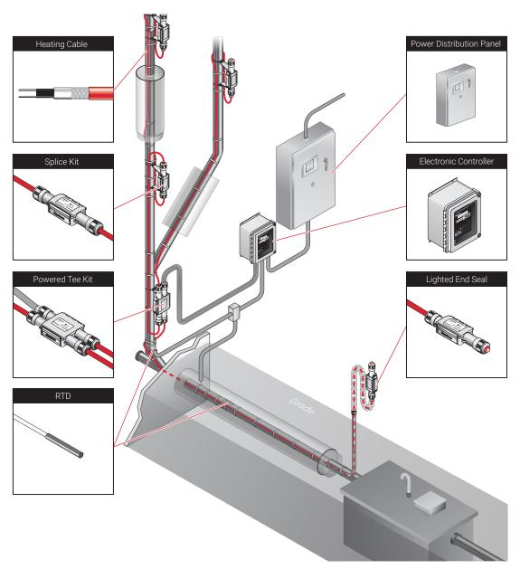
Fig. 6 Typical XL-Trace flow maintenance system
