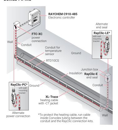
Fig. 5 Typical buried piping system
