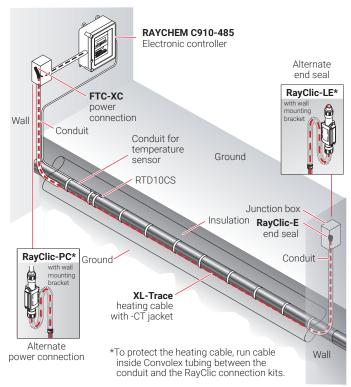
Fig. 14 Typical buried piping system
