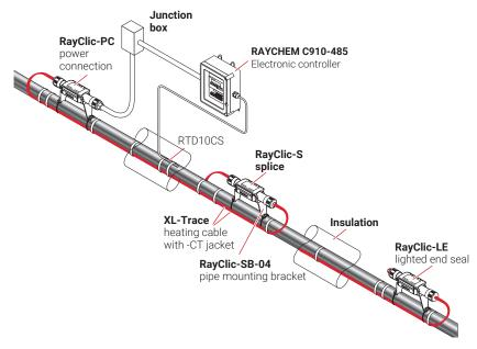
Fig. 9 Typical aboveground piping system
