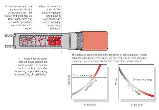
Fig. 2 Self-regulating heating cable technology
