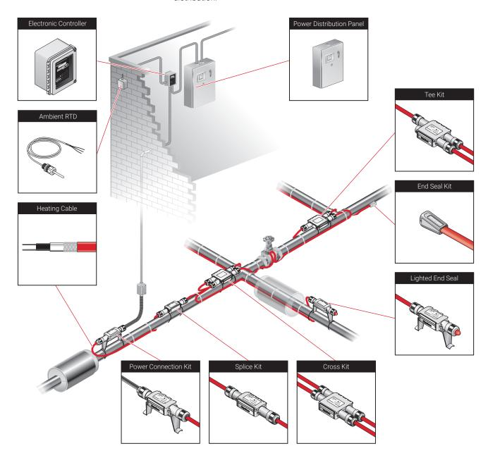
Fig. 3 Typical XL-Trace pipe freeze protection system
