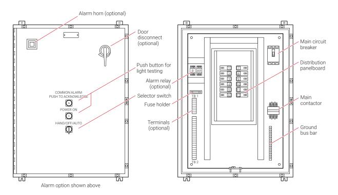
Fig. 16 HTPG power distribution panel
