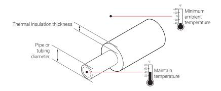
Fig. 10 Pipe heat loss
