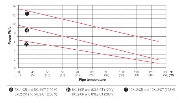
Fig. 12 Heating cable power output on metal pipe
