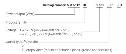
Fig. 11 Heating cable catalog number
