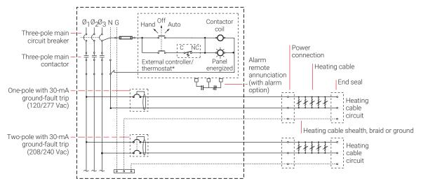
Fig. 17 HTPG power schematic
