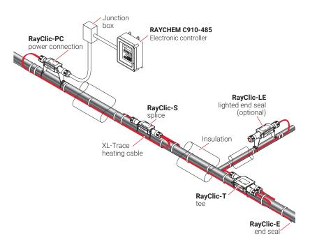
Fig. 4 Typical aboveground piping system
