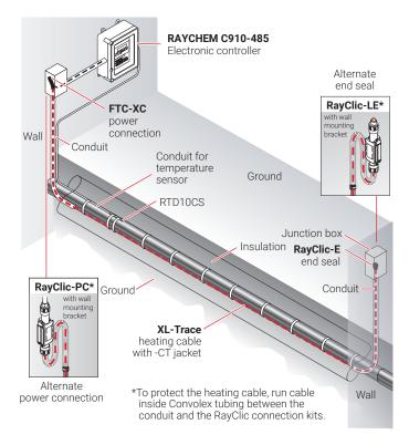
Fig. 8 Typical buried grease waste line
