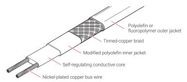
Fig. 1 XL-Trace heating cable construction
