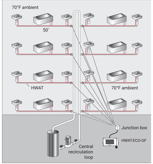
Fig. 1 Generic hybrid HWAT system
