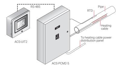
Fig. 6 Typical configuration for the ACS-30 system
