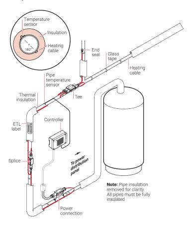
Fig. 1 Typical HWAT heating cable system
