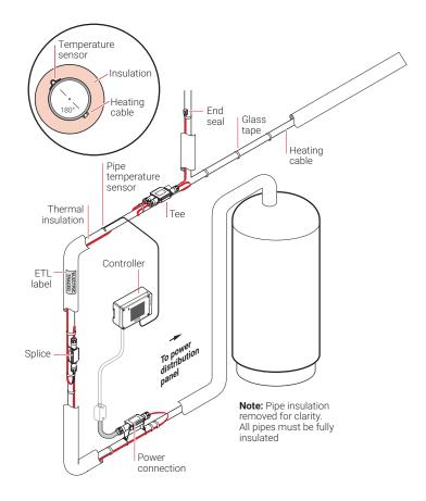
Fig. 5 Typical HWAT heating cable system
