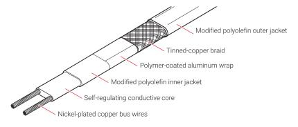
Fig. 3 HWAT-R2 heating cable
